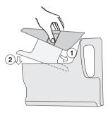
■ After cleaning, dry both parts thoroughly before replacing it in the water container. When replacing the insert (see illustration), guide it in at an angle ① and push the side with the opening downwards ②.
